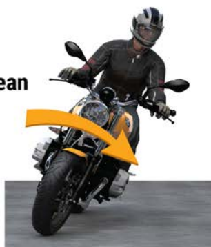
Front wheel momentarily out-tracks away from turn, causing motorcycle to begin leaning in turn direction.
