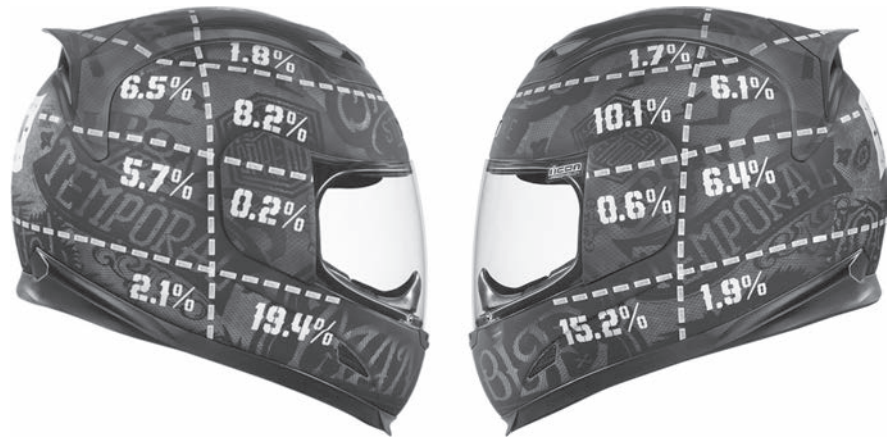
Distribution of Impact Locations on Motorcycle Helmets; All Collisions based on a study by Dietmar Otte.
